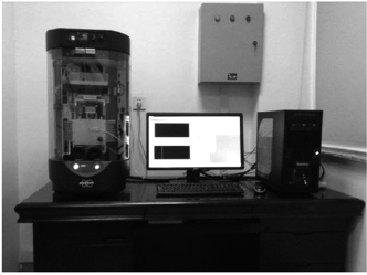
图 1 高温摩擦磨损实验设备 Fig. 1 High temperature friction-wear test equipment
