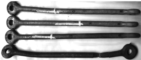
图 1 更换的延长拉杆图片 Fig. 1 Image of replaced extension rod
