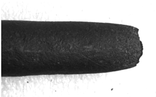
图 2 断裂延长拉杆断口附近形貌 Fig. 2 Morphology near fracture of fractured extension rod
