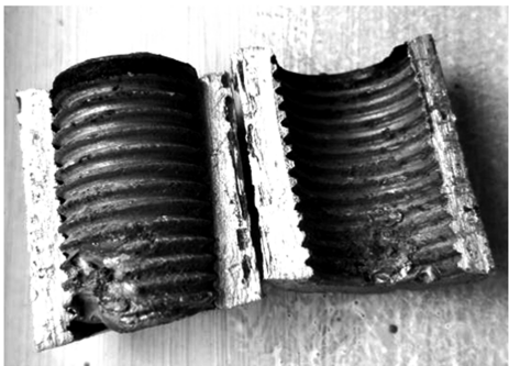
图 4 支撑杆局部熔化形貌 Fig. 4 Local melting morphology of support rod
