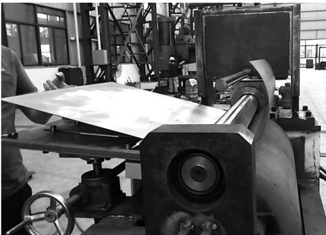
图 4 TC4 钛合金两轴柔性滚弯试验装置 Fig. 4 Test device of two-axe flexible roll bending for TC4 titanium alloy
