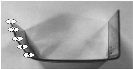
图 9 SUS430 不锈钢自由曲面弯曲成形件测量点选取 Fig. 9 Selection of measurement points for free-form surface bending part of SUS430 stainless steel
