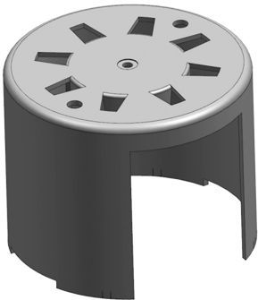
图2 步进电机外壳零件3D图 Fig. 2 3D drawing of stepper motor shell parts
