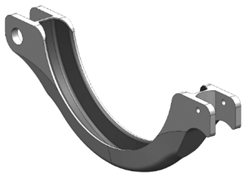
图 1 卡箍模座零件的三维形状示意图 Fig. 1 Schematic diagram of three-dimensional shape for clamp mold base part
