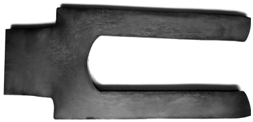
图 12 成形锻件金属流线分布 Fig. 12 Distribution of metal streamline for formed forgings
