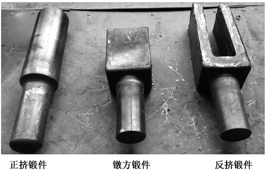
图 11 改进成形工艺各工序的成形锻件 Fig. 11 Forgings formed by each process of improved forming process
