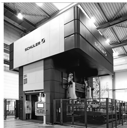
图4 德国舒勒公司采用 PCH 热冲压工艺技术的成形装备 Fig. 4 Forming equipment using PCH hot stamping process technology of Schuler company in Germany
