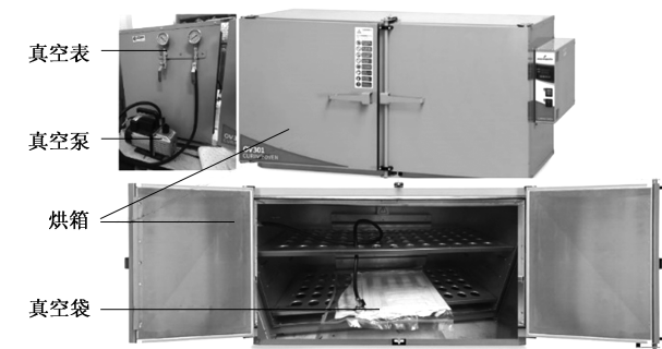
图 2 真空固化工艺试验设备 Fig. 2 Test equipment of vacuum curing process
