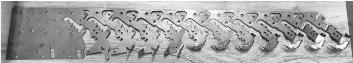
图 7 产品料带图 Fig. 7 Drawing of product strip
