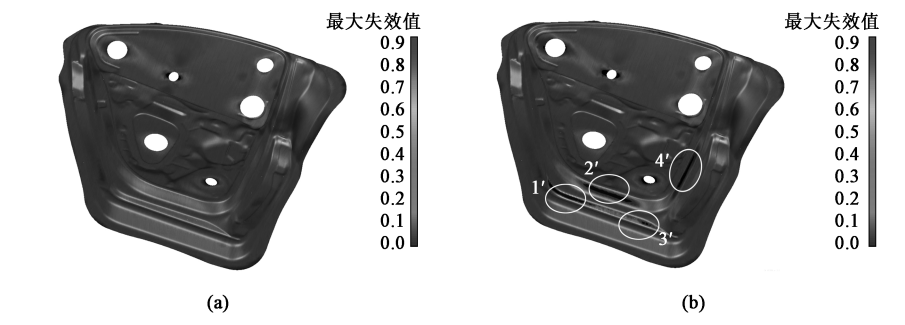
图 12 2#门内板最大失效对比 (a) Nominal 模式下失效区域 (b) Sigma 模式下失效区域 Fig. 12 Comparison of maximum failure for 2# door inner panel (a) Failure area in Nominal mode (b) Failure area in Sigma mode
