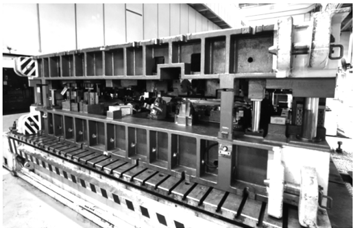
图 9 尾门内外板上模倾斜问题解决 Fig. 9 Solving of deflection problem of upper die for tailgate inner and outer panels
