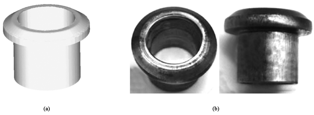
图 13 模具改进后模拟件与试验件成形情况对比 (a) 模拟件 (b) 试验件 Fig. 13 Comparison of forming conditions between simulated and tested parts after die improvement (a) Simulated part (b) Tested part
