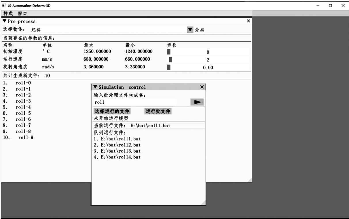
图 3 DEFORM-3D 自动化前处理程序 Fig. 3 DEFORM-3D automatic pre-processing program
