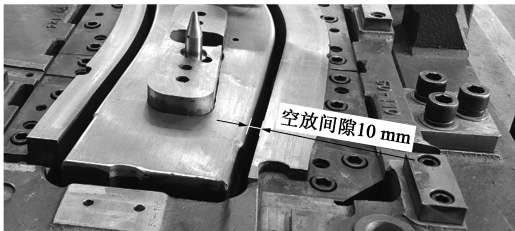
图 7 压料翻边成形空开设计 Fig. 7 Open design in pressing and flanging
