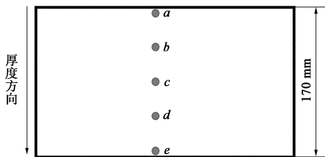
图 3 力学性能检验时 45 钢复合板厚度方向不同位置的取样示意图 Fig.3 Schematic diagram of sampling at different positions along thickness direction of 45 steel composite plate for mechanical properties test
