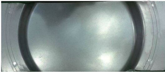
图 1 一次加载抗凹试样 Fig. 1 Dent resistance specimen by one-time loading
