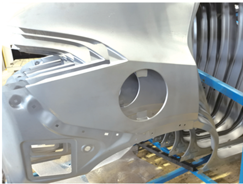
图 10 侧围外板生产验证 Fig. 10 Production verification of side wall outer panel
