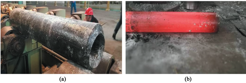
图 2 挤压获得的厚壁钢管 (a) 挤压后的钢管 (b) 冷却后的钢管 Fig. 2 Extruded thick-walled steel pipe (a) Extruded steel pipe (b) Cooled steel pipe
