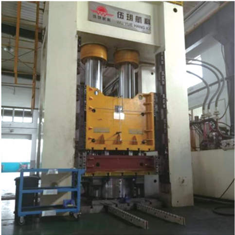
图 11 800 t 充液成形设备图 Fig. 11 Diagram of 800 t hydroforming equipment
