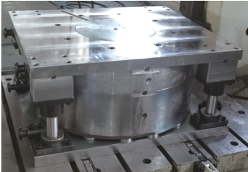
图 10 立式内高压胀形模具实物图 Fig. 10 Physical picture of vertical internal high-pressure bulging die
